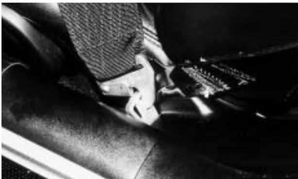
**3** The Brey-Krause kit is designed to use lap belts with a clip-in installation. This means they can be unsnapped in seconds and safely stored out of the way when not in use.
