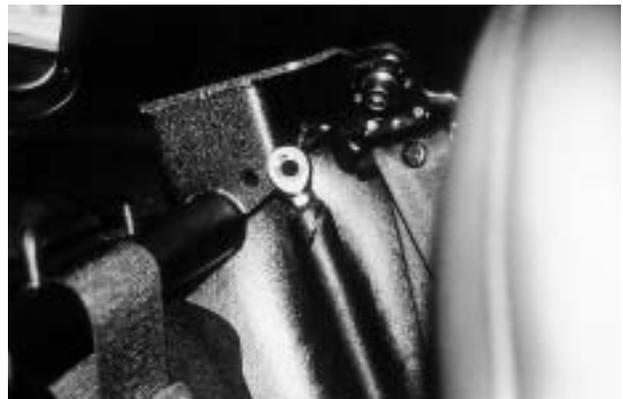
**6** The support rod uses the rear-seat bolt to fasten it to the floor, and the upper bolt holds it solidly to the harness bar.
