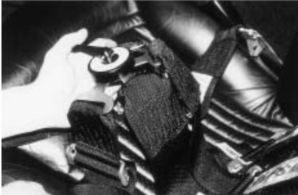
**7** We contacted Simpson Race Products for the necessary harnesses for this application. There are several color options available, with either a cam-lock fastener or the latch-link system. We opted for the cam-lock.
