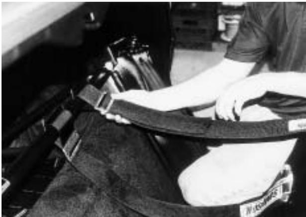
**8** The wraparound mounting utilizes a buckle that allows for a broad range of adjustment.
